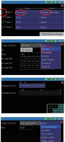
Back to the trigger setting display by "Esc" and touch "Action" of the trigger 0, then select "Stop Measurement". e.g.: Output a pulse to the external device when receiving a specific error.
