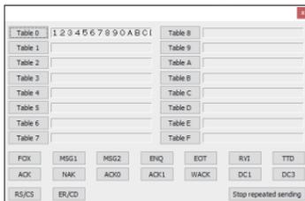
When "Repeat" function is ON, data corresponding to the data table will be transmitted continuously spacing for idle time.
