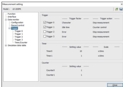
Up to four triggers can be set. Trigger factor and action can be set for each trigger independently. Each trigger can be set either to be enable or disable.
