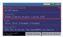
Measurement port / : Select a measurement port of line monitor and a function.
