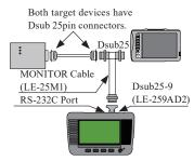
Connect the target devices and the line monitor using the optional Dsub25-9pin adapter (LE-259AD2) and Dsub25pin monitor cable (LE-25M1).
