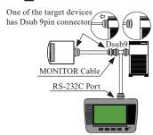
Connect the target devices and the line monitor using the included monitor cable (LE-009M2)
