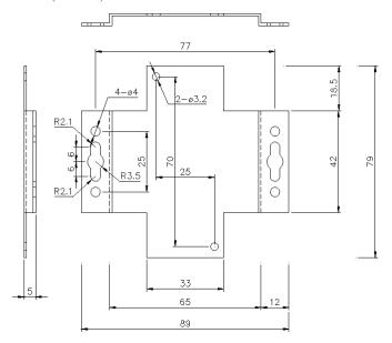
Two  $\phi 3.2$  holes are for attaching this bracket on the backside of the converter, other holes on each side of the bracket are for attaching on the wall.
