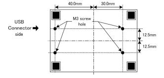
Notice: Use the screws that can be inserted less than 6mm from the surface line. If it is inserted deeper, it may damage the circuit.
