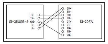
An example of N:N connection between RS-485 devices (between SI-35USB-2)
