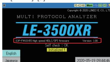
Save your important data in the SD cards before changing the firmware mode. It will initialize the analyzer and erase all data when the analyzer changes the measuring mode.
