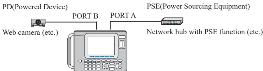
Connection to PORT A and PORT B are compatible.
