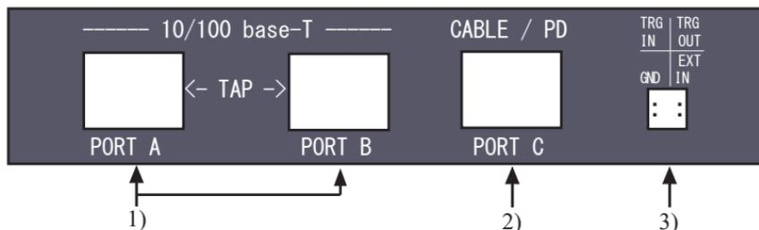
1)PORT A, B For on-line monitor, PoE measurement, Statistic analysis (Fail-safe TAP for PoE devices), PING function, and Port blinking function (LAN ports of 10BASE-T/100BASE-TX).
