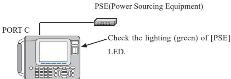
When connecting "PSE" and "Port A", "Port B" and "Port C" as following, it is able to know more intimate analysis on PSE powering type, voltage and so on. In this case, the PD on Port C is measured with approximately 4.7kΩ of load.
