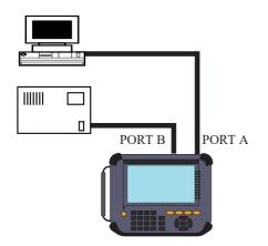
Delay is occurred when it passes through the TAP circuit in the analyzer.
