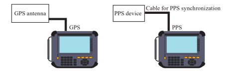
To use one GPS active antenna and synchronize 2 sets of LE-8600X/LE-8500X, connect devices as following.
