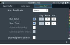
Set the automatic measurement period for "Run time" and "Stop time"
