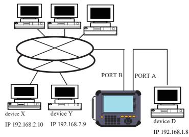
• Monitoring example of TCP/IP frames between Device A and D by filtering.
