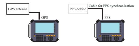
To use one GPS active antenna and synchronize 2 sets of LE-8500X, connect devices as following.
