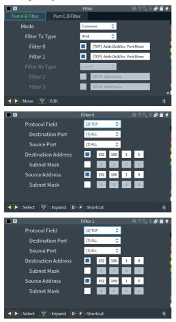
The filter 0 is configured to monitor TCP frames sent from the device D to device A and the filter 1 is configured to monitor TCP frames sent from the device A to device D. Configures this setting between port A-B.
