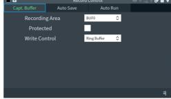
Select Ring buffer (endless recording) or Full stop when the capture buffer is full.
