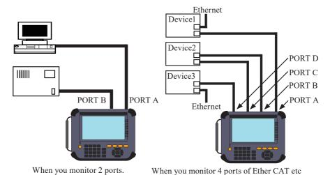
Delay is occurred when it passes through the TAP circuit in the analyzer.
