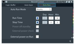
Set the automatic measurement period for "Run time" and "Stop time"
