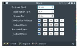
It is configured by filter 4 to monitor only the frames of UDP protocol which have "192.16.2" for the network address part of both source IP and destination IP.
