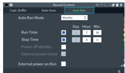
Set the automatic measurement period for "Run time" and "Stop time"
