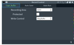
Select Ring buffer (endless recording) or Full stop when the capture buffer is full.
