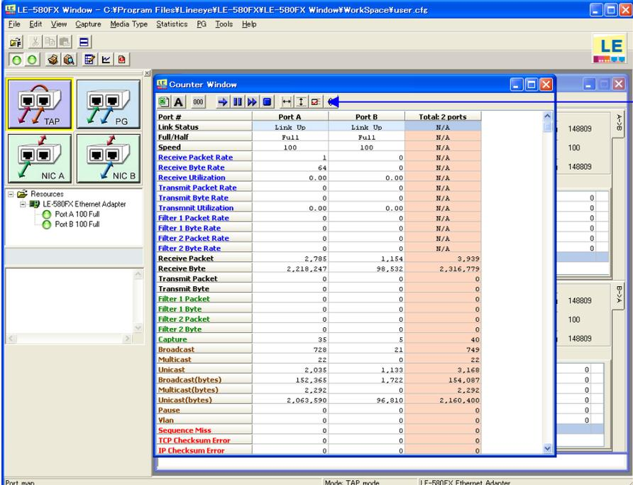
Control bar to clear/start/stop counter and adjust counter alignment/size.
