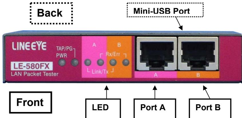
Mini-USB port : to connect with PC by Mini-USB cable.
