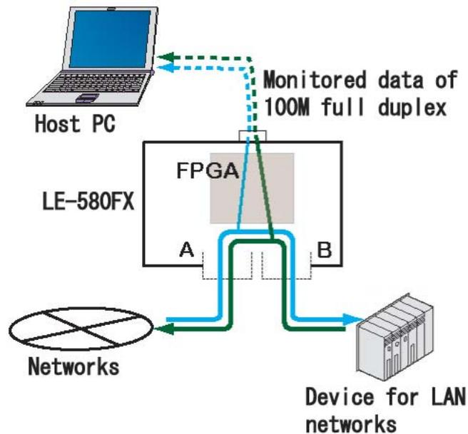
\*When either A or B port of LE-580FX is connected to LAN cable, LE-580FX is in NIC mode. And when both A and B port of LE-580FX are connected to LAN cables, LE-580FX is in TAP mode.
