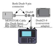
If the connectors of both target devices are Dsub 9 pin, use attached Dsub 9 pin monitor cable (LE-009M2) and Dsub 25-9 conversion adapter to connect to the analyzer.
