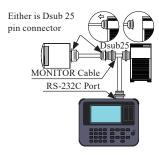
If the connector of either target device is Dsub 25 pin, use attached Dsub 25 pin monitor cable (LE-25M1) to connect to the analyzer.
