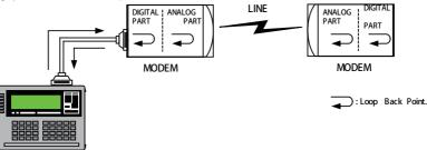
The loop-back point can be usually set and changed by using the self-test function of the modem. (Refer to the instruction manual of the modem.)
